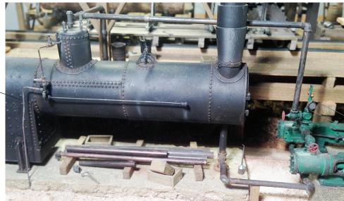
Water Supply Line This line connects to the open bore on the injector and connects to the water supply. In this case it drops into the ground. This detail is denoted "c" in the drawing.
